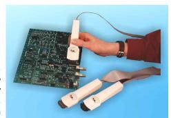
The Advanced Test Module is equally at ease with testing large quantities of boards (production testing) and testing in-circuit single components (repair and diagnostics).
